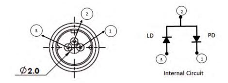
1. PD Cathode; 2. COM (LD Cathode, PD Anode); 3. LD Anode
