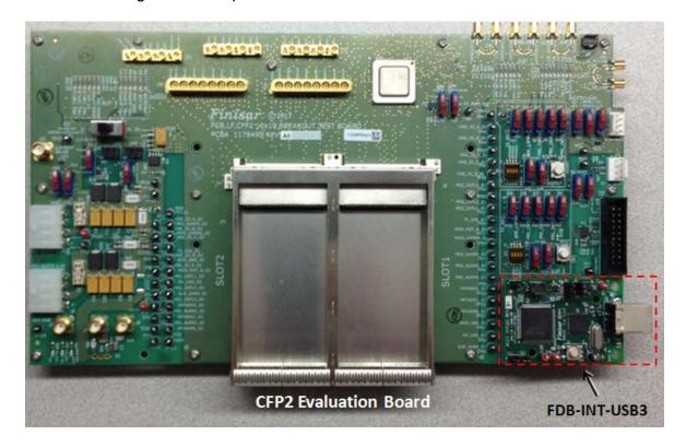
The FDB-INT-USB3 is used with the FDB-1032-SFP+ evaluation board (for SFP/SFP+/SFP28 transceivers) as shown below in the red-dashed rectangle on the top side of the board:
